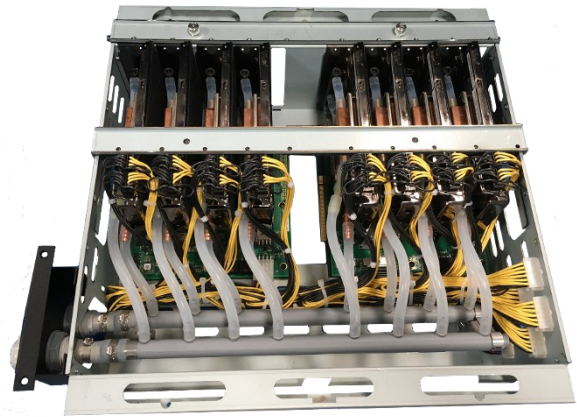
Chillydyne GPU System with Internal Server Manifold
