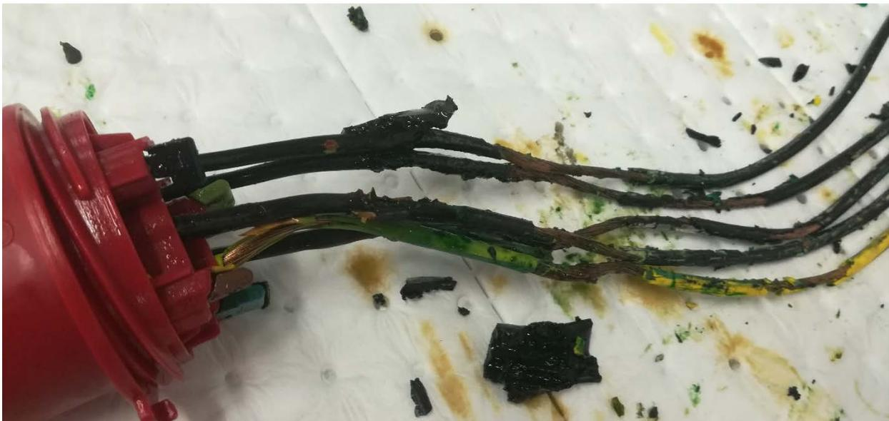
*Figure 1: Oil Immersion image (Power cable after wicking oil from oil bath.)<sup>2</sup>*
