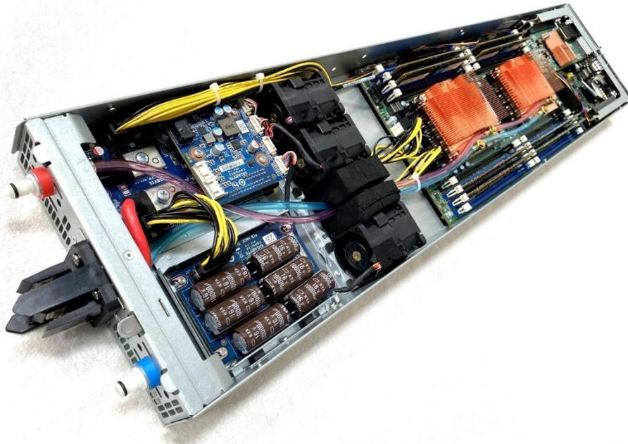
*Figure 2 Relion server with two Xeon Gold processors with Cool-Flo™ hybrid liquid-air heat sinks*
